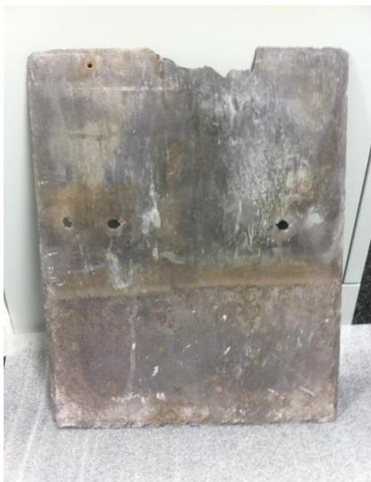
Photo of a reclaimed slate. The slate has already been re-fixed at least one in its life. The second set of nail holes are too close to the centre. This slate should **NOT** be reused.
